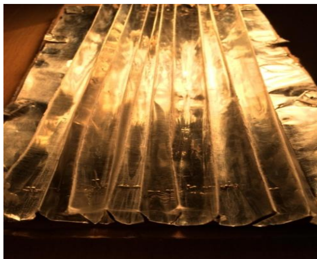
Figure 6e: Design Electrospinning Setup (zigzag aluminum collector)
