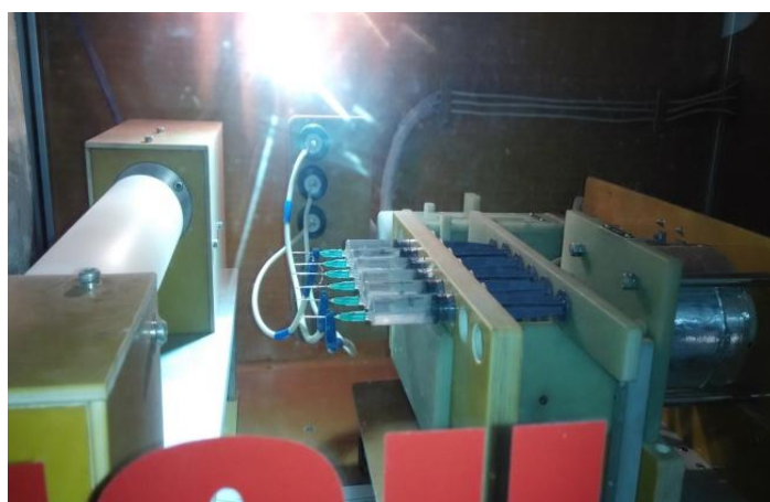
figure 7 b: Electrospinning Setup
