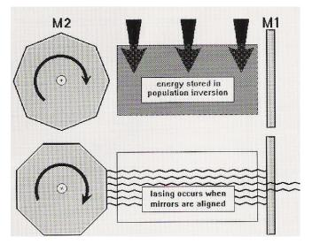
Shorter duration pulses are obtained with Qswitching. A simple Q -switch uses a mirror as part of the optical cavity. Only when the rotating mirror is precisely aligned with the output mirror is lasing possible, so lasing is restricted to a very short time interval (1-10 seconds). Between alignments, energy is stored in the excited population. Thus several hundred mili joules of energy can be squeezed into nano second pulses.
