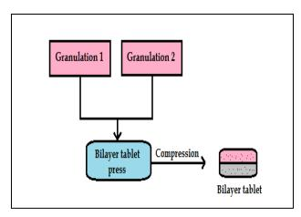
Figure 6: The basic concept of Bilayer tablets
