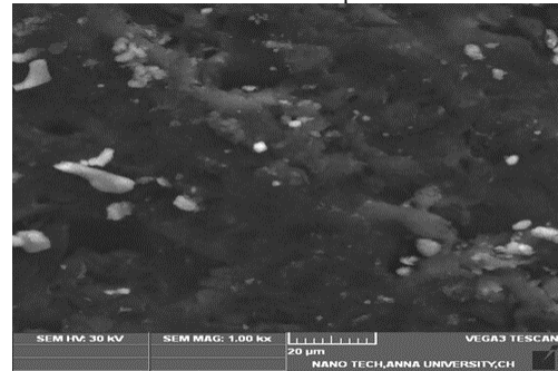
Figure 7: SEM image of provisional PMMA reinforced with 2.5% Alumina nanoparticles
