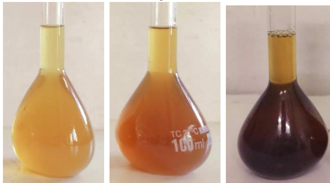
Figure 1: Colour changes observed during the synthesis of zinc oxide nanoparticles
