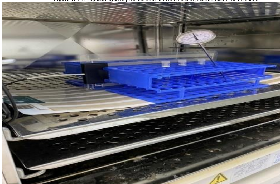
Figure 1: The exposure system presents tubes and antennas in position inside the incubator
