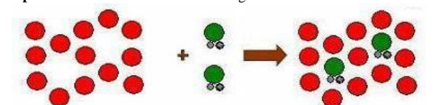
Step 3: The freed solid molecule is integrated into the hole in the solvent
