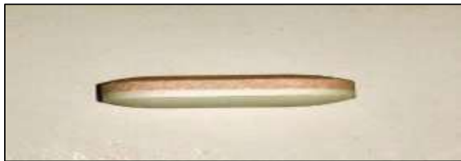
Figure 8: Bilayer tablets comprising different APIs (Heterogeneous)
