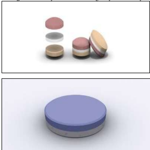
Figure 5: Multilayered tablets showing trilayered and bilayer tablets
